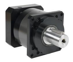
LS Electric high-precision planetary gearbox, 5:1 ratio, inline, 55mm diameter output shaft, nominal output torque 1195 N-m (10577 lb-in), 1-stage, 180mm frame. For use with APM-FF series 7.5 kW motors.
