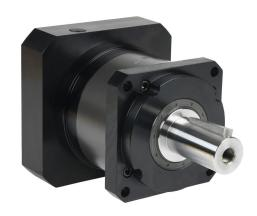
LS Electric high-precision planetary gearbox, 10:1 ratio, inline, 40mm diameter output shaft, nominal output torque 500 N-m (4426 lb-in), 1-stage, 142mm frame. For use with APM-FF series 3.5 kW and 5.5 kW motors.
