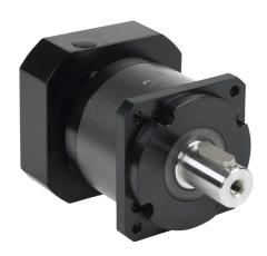
LS Electric high-precision planetary gearbox, 10:1 ratio, inline, 32mm diameter output shaft, nominal output torque 262 N-m (2319 lb-in), 1-stage, 115mm frame. For use with APM-FE series 2.2 kW motors.
