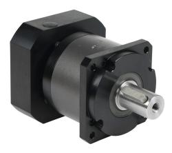
LS Electric high-precision planetary gearbox, 5:1 ratio, inline, 32mm diameter output shaft, nominal output torque 332 N-m (2939 lb-in), 1-stage, 115mm frame. For use with APM-FE series 2.2 kW motors.
