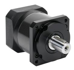
LS Electric high-precision planetary gearbox, 10:1 ratio, inline, 22mm diameter output shaft, nominal output torque 121 N-m (1071 lb-in), 1-stage, 90mm frame. For use with FCL series 750W and 1 kW motors.
