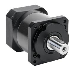
LS Electric high-precision planetary gearbox, 5:1 ratio, inline, 22mm diameter output shaft, nominal output torque 160 N-m (1416 lb-in), 1-stage, 90mm frame. For use with FCL series 750W and 1 kW motors.
