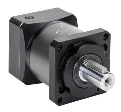
LS Electric high-precision planetary gearbox, 10:1 ratio, inline, 16mm diameter output shaft, nominal output torque 42 N-m (372 lb-in), 1-stage, 60mm frame. For use with FBL series 100W, 200W and 400W motors.
