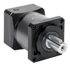
LS Electric high-precision planetary gearbox, 10:1 ratio, inline, 16mm diameter output shaft, nominal output torque 42 N-m (372 lb-in), 1-stage, 60mm frame. For use with FBL series 100W-400W motors.
