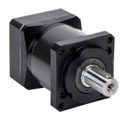
LS Electric high-precision planetary gearbox, 5:1 ratio, inline, 16mm diameter output shaft, nominal output torque 54 N-m (478 lb-in), 1-stage, 60mm frame. For use with FBL series 100W, 200W and 400W motors.
