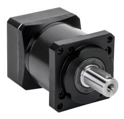
LS Electric high-precision planetary gearbox, 5:1 ratio, inline, 16mm diameter output shaft, nominal output torque 54 N-m (478 lb-in), 1-stage, 60mm frame. For use with FBL series 100W-400W motors.
