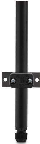
WERMA mounting tube with clamp, 25mm diameter, 250mm length, black, polyamide. For use with 70mm terminal elements. M16 x 1.5mm cable gland included.
