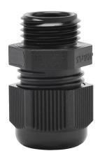
WERMA cable gland, M16 x 1.5mm thread type, polyamide, black, accepts 5 to 10mm diameter cable, IP68.
