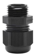
WERMA cable gland, M16 x 1.5mm thread type, polyamide, black, accepts 5 to 10mm diameter cable, IP68.
