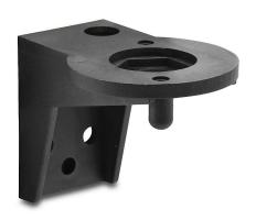
WERMA mounting bracket, surface mount, black, polyamide. For use with 70mm terminal elements. M16 x 1.5mm cable gland included.
