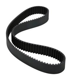
SureMotion timing belt, 8mm 8M pitch, 30mm wide, 120 tooth, 960mm pitch length (circumference), neoprene, fiberglass reinforced.
