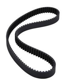
SureMotion timing belt, 8mm 8M pitch, 20mm wide, 120 tooth, 960mm pitch length (circumference), neoprene, fiberglass reinforced.
