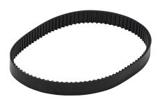
SureMotion timing belt, 0.08in MXL pitch, 1/4in wide, 95 tooth, 7.6in pitch length (circumference), polyurethane, polyester reinforced. Package of 3.
