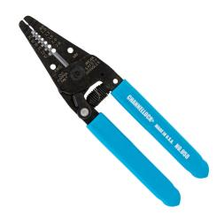
CHANNELLOCK multi-purpose wiring tool, compatible with data & communications cable and round wire, precision machined hardened cutting edges, 20-12 AWG stranded and 18-10 AWG solid wire stripping capacity, 10 AWG cutting capacity.
