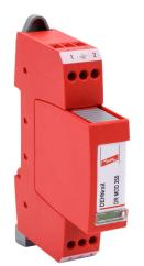
Dehn DR-M-2P series supplemental power & controls Surge Protective Device (SPD), 3 kA discharge current, 230VAC/DC 1-Phase, series or parallel circuit, 35mm DIN rail mount.
