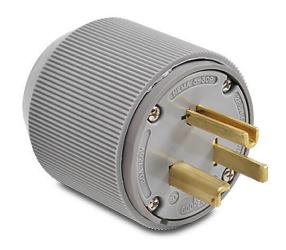
Bryant industrial heavy duty straight blade plug, 30A, 125 VAC, 1-phase, 2-pole, 3-wire, NEMA 5-30, accepts cord size 0.42-1.32in, thermoplastic housing, gray.
