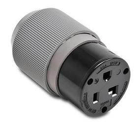
Bryant industrial heavy duty straight blade connector, 30A, 125 VAC, 1-phase, 2-pole, 3-wire, NEMA 5-30, accepts cord size 0.42-1.32in, thermoplastic housing, gray.
