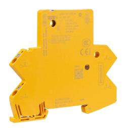
Dehn BCO compact series data & signal Surge Protective Device (SPD), 5 kA discharge current, 5 VAC/VDC, series circuit, indirect grounding, 2 lines or 1 pair, 35mm DIN rail mount.
