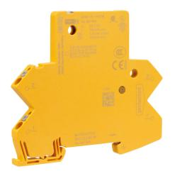
Dehn BCO compact series data & signal Surge Protective Device (SPD), 5 kA discharge current, 24 VAC/VDC, series circuit, indirect grounding, 2 lines or 1 pair, 35mm DIN rail mount.
