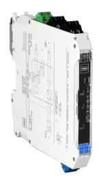
STAHL ISpac intrinsically safe digital output isolator, 15-30 VDC input, 48 mA at 9.7 VDC output, 24 VDC operating voltage, screw terminals.
