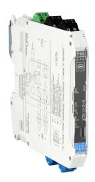
STAHL ISpac intrinsically safe digital input isolator, (2) NAMUR sensors or (2) dry contacts input, (2) N.O. contacts output, 24 VDC operating voltage, screw terminals.
