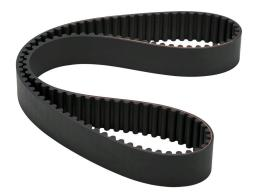
SureMotion timing belt, 8mm 8M pitch, 30mm wide, 115 tooth, 920mm pitch length (circumference), neoprene, fiberglass reinforced.
