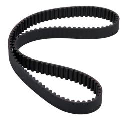
SureMotion timing belt, 8mm 8M pitch, 20mm wide, 115 tooth, 920mm pitch length (circumference), neoprene, fiberglass reinforced.
