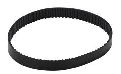
SureMotion timing belt, 0.08in MXL pitch, 1/4in wide, 91 tooth, 7.3in pitch length (circumference), polyurethane, polyester reinforced. Package of 3.
