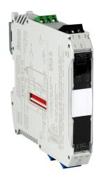
STAHL ISpac intrinsically safe temperature input isolator, RTD or thermocouple input, 0-20 mA or 4-20 mA output, 24 VDC operating voltage, screw terminals.
