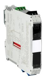
STAHL intrinsically safe temperature input isolator, RTD or thermocouple input, 0-20 mA or 4-20 mA output, 24 VDC operating voltage.
