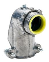
Halex fitting, zinc die cast, 90-degree, 3/4in trade size, screw clamp conduit connection, insulation. Package of 10. For use with flexible metal conduit (FMC), AC cable (BX), MC cable. Screws and locknut included.
