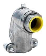
Halex fitting, zinc die cast, 90-degree, 1/2in trade size, screw clamp conduit connection, insulation. Package of 25. For use with flexible metal conduit (FMC), AC cable (BX), MC cable. Screws and locknut included.
