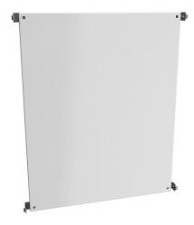
Hammond subpanel, half-height, carbon steel, RAL 9003 white, powder coat finish. For use with 90x36 (HxW) 1418YYxx and HN4FS9036xxxx freestanding enclosures.
