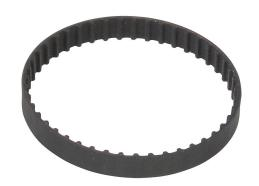
SureMotion timing belt, 1/5in XL pitch, 3/8in wide, 45 tooth, 9in pitch length (circumference), neoprene, fiberglass reinforced.
