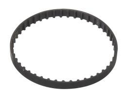
SureMotion timing belt, 1/5in XL pitch, 1/4in wide, 45 tooth, 9in pitch length (circumference), neoprene, fiberglass reinforced.
