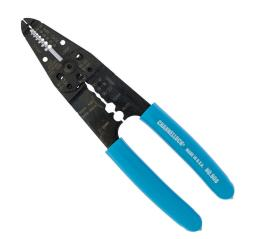
CHANNELLOCK multi-purpose wiring tool, compatible with data & communications cable and round wire, precision machined hardened cutting edges, 22-12 AWG stranded and 20-10 AWG solid wire stripping capacity, 10 AWG cutting capacity.
