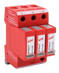
Dehn DG-MU series power Surge Protective Device (SPD), 20 kA discharge current, 480 VAC 3-Phase Delta, parallel circuit, 35mm DIN rail mount.
