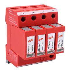
Dehn DG-MU series power Surge Protective Device (SPD), 20 kA discharge current, 600/347 VAC 3-Phase Wye, neutral ground protection, parallel circuit, 35mm DIN rail mount.
