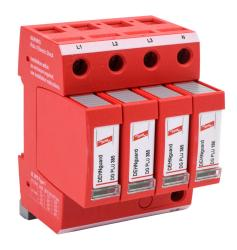
Dehn DG-MU series power Surge Protective Device (SPD), 20 kA discharge current, 480/277 VAC 3-Phase Wye, neutral ground protection, parallel circuit, 35mm DIN rail mount.
