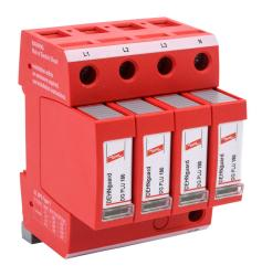
Dehn DG-MU series power Surge Protective Device (SPD), 20 kA discharge current, 208/120 VAC 3-Phase Wye, neutral ground protection, parallel circuit, 35mm DIN rail mount.
