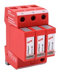
Dehn DG-MU series power Surge Protective Device (SPD), 20 kA discharge current, 480/277 VAC 3-Phase Wye, parallel circuit, 35mm DIN rail mount.
