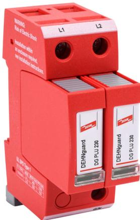
Dehn DG-MU series power Surge Protective Device (SPD), 20 kA discharge current, 240/120 VAC Split Phase, parallel circuit, 35mm DIN rail mount.
