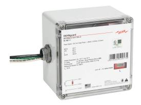
Dehn EZ50-S series power Surge Protective Device (SPD), 20 kA discharge current, 120 VAC 1-Phase, parallel circuit, NEMA 4X enclosure rating, IP66, 1/2in NPSM/Wall mount.
