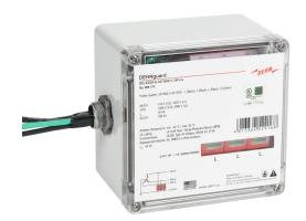
Dehn EZ50-S series power Surge Protective Device (SPD), 20 kA discharge current, 600/347 VAC 3-Phase Wye, parallel circuit, NEMA 4X enclosure rating, IP66, 1/2in NPSM/Wall mount.
