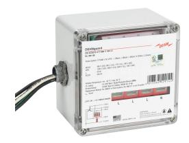
Dehn EZ50-S series power Surge Protective Device (SPD), 20 kA discharge current, 480/277 VAC 3-Phase Wye, neutral ground protection, parallel circuit, NEMA 4X enclosure rating, IP66, 1/2in NPSM/Wall mount.
