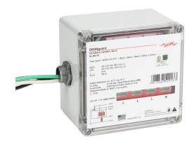
Dehn EZ50-S series power Surge Protective Device (SPD), 20 kA discharge current, 208/120 VAC 3-Phase Wye, neutral ground protection, parallel circuit, NEMA 4X enclosure rating, IP66, 1/2in NPSM/Wall mount.
