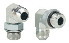
HY-TECH hydraulic fluid adapter, elbow, plated steel body, (1) -8 male JIC 37 deg and (1) -8 male o-ring boss. Package of 2.
