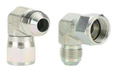
HY-TECH hydraulic fluid adapter, elbow, plated steel body, (1) -8 male JIC 37 deg and (1) -8 female JIC 37 deg. Package of 2.
