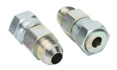
HY-TECH hydraulic fluid adapter, straight, plated steel body, (1) -8 male JIC 37 deg and (1) -8 female flat face o-ring. Package of 2.
