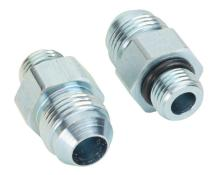
HY-TECH hydraulic fluid adapter, straight, plated steel body, (1) -8 male JIC 37 deg and (1) -6 male o-ring boss. Package of 2.
