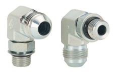
HY-TECH hydraulic fluid adapter, elbow, plated steel body, (1) -8 male JIC 37 deg and (1) -6 male o-ring boss. Package of 2.
