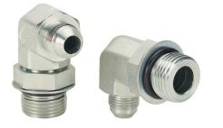
HY-TECH hydraulic fluid adapter, elbow, plated steel body, (1) -8 male JIC 37 deg and (1) -12 male o-ring boss. Package of 2.
