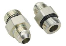
HY-TECH hydraulic fluid adapter, straight, plated steel body, (1) -8 male JIC 37 deg and (1) -10 male o-ring boss. Package of 2.
