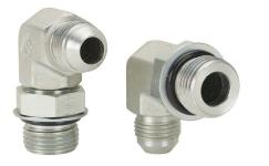
HY-TECH hydraulic fluid adapter, elbow, plated steel body, (1) -8 male JIC 37 deg and (1) -10 male o-ring boss. Package of 2.
